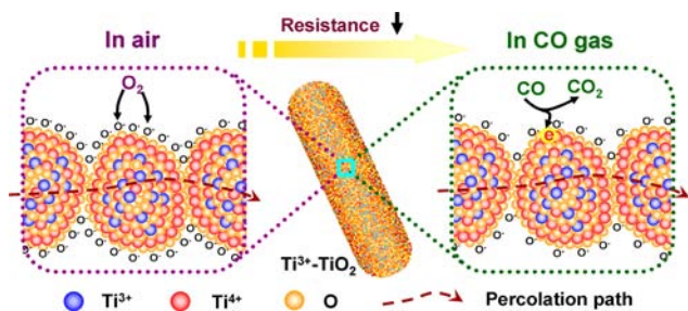
Figure 9. Schematic representation of the sensing mechanism of Ti 3+ -TiO 2 . Resistance ↓ means resistance decrease. Percolation path means electron transport pathway between the Au electrodes of the sensor.
